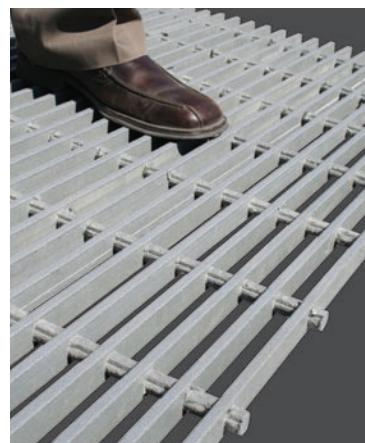
DURAGRID® R-7300 1" fiberglass grating weighs only 3.2 lbs. per square foot, less than half the 7.4 lbs. per square foot for 1" steel grating. The fiberglass grating will also span 36" with a load of 100 lbs. per square foot resulting in deflection of less than 1/4".
