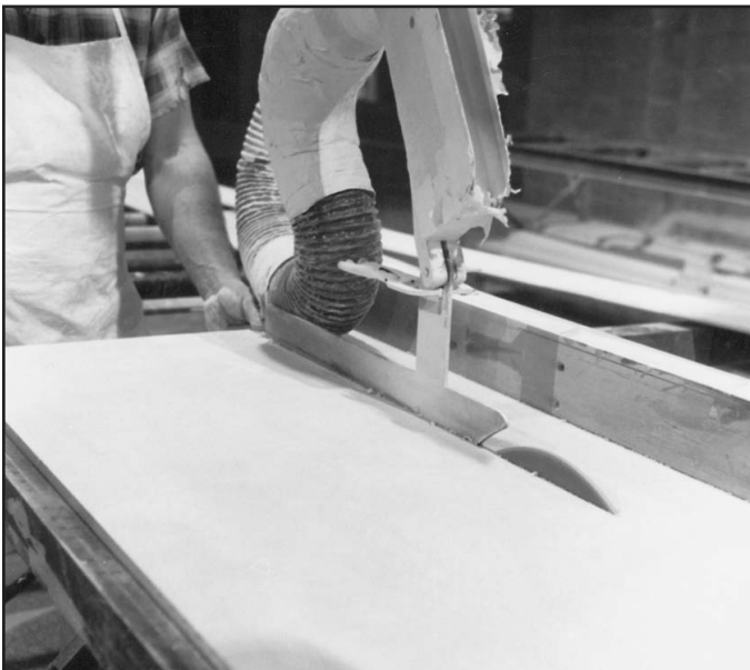
Straight line sawing (vacuum hood raised).
