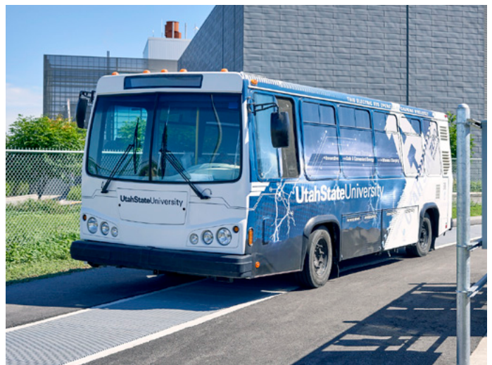
HD-4000 2-1/2" was used as a trench cover to protect wireless electromagnetic charging devices built into the roadway at the Utah State University Electric Vehicle and Roadway research facility in Logan, Utah.
