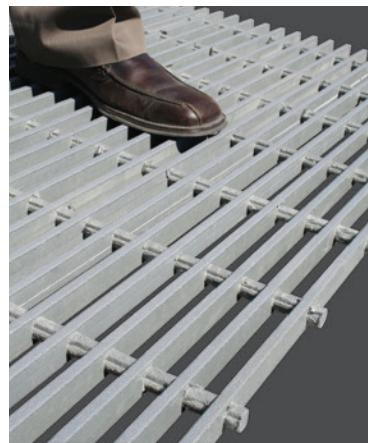
DURAGRID® R-7300 1" fiberglass grating weighs only 3.2 lbs. per square foot, less than half the 7.4 lbs. per square foot for 1" steel grating. The fiberglass grating will also span 36" with a load of 100 lbs. per square foot resulting in deflection of less than  $\frac{1}{4}$ ".
