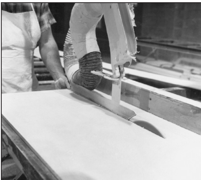
Straight line sawing (vacuum hood raised).
