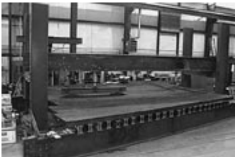
Figure 30. Full scale mock-up of Tom's Creek Bridge.
