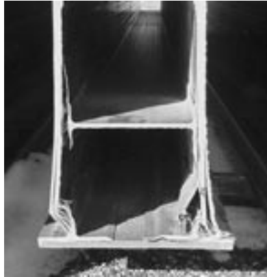
Figure 15: Bearing failure at supports for 36" DWB tested at L/d of 6.
