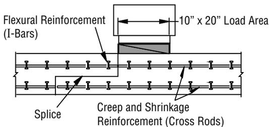
DESIGNING WITH GRIDFORM™: The University of Wisconsin has developed software for designing decks reinforced with GRIDFORM™. The program is capable of computing bridge deck capacity including ultimate capacities of flexure, punching shear and flexural shear. Serviceability issues (i.e. slab deflection and crack width) is also incorporated into the design aid, available on Strongwell.com.
