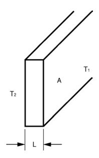
$$Q = kA \frac{\Delta T}{L} = \frac{\Delta T}{R} A = \frac{T_2 - T_1}{R} A$$
