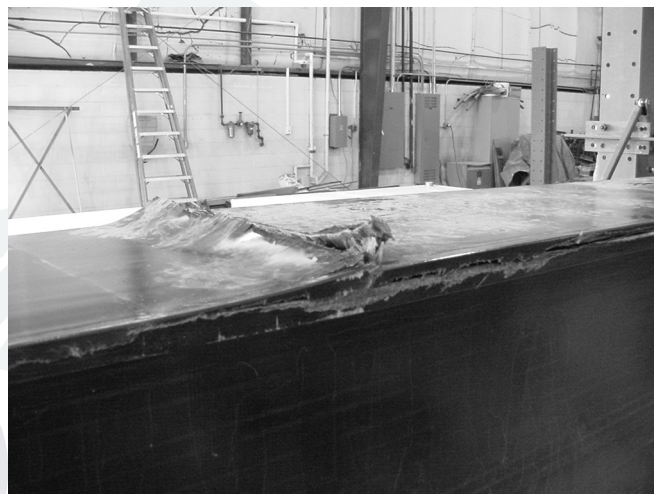
Figure 13: Typical compression flange failures for four point bend testing of the 8" DWB (top photo) and the 36" DWB (bottom photo).
