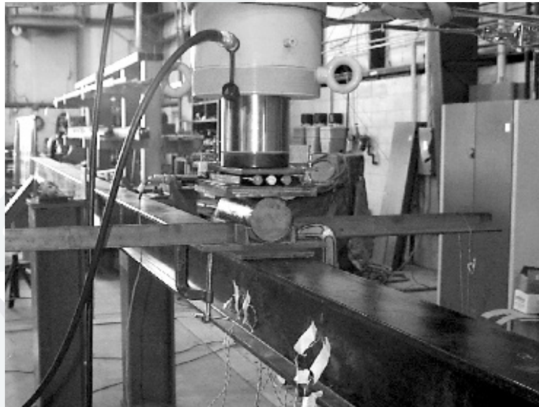
Figure 7: Loading point configuration to allow rotation and translation of the midspan.
