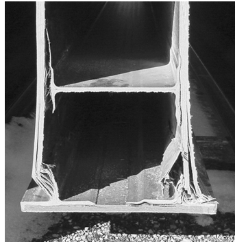
Figure 14: Bearing failure at supports for 36" DWB tested at L/d of 6.
